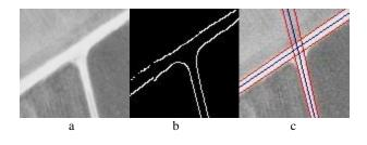
Figure 6: Three-arm junction: a) original image, b) edges, c) detected straight lines (red) and the computed centerline (blue)
