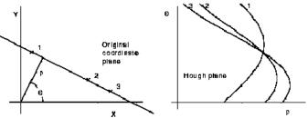
Figure 1: The coordinate system of the original image and the Hough-space [1]
