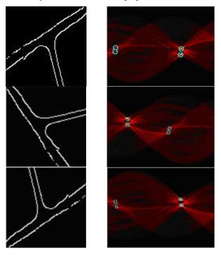
Figure 7: Rotated (0° - 90° - 180°) road edges and the Radonspace.
