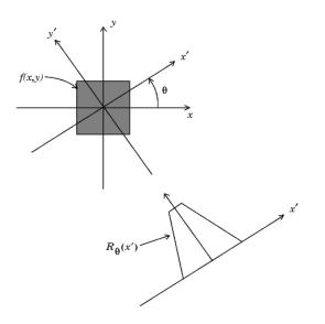
Figure 2: The original image and its projection [4]
