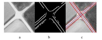
Figure 5: Four-arm junction: a) original image, b) edges, c) detected straight lines (red) and the computed centerline (blue)
